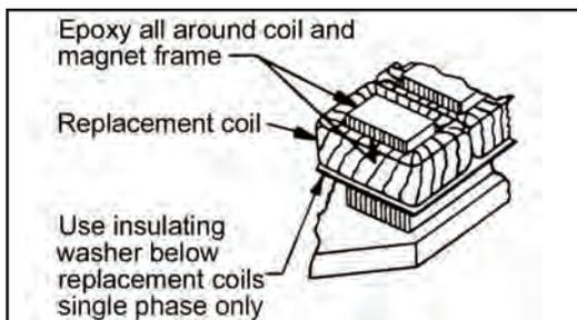
Figure 3. Fastening of Replacement Magnet
